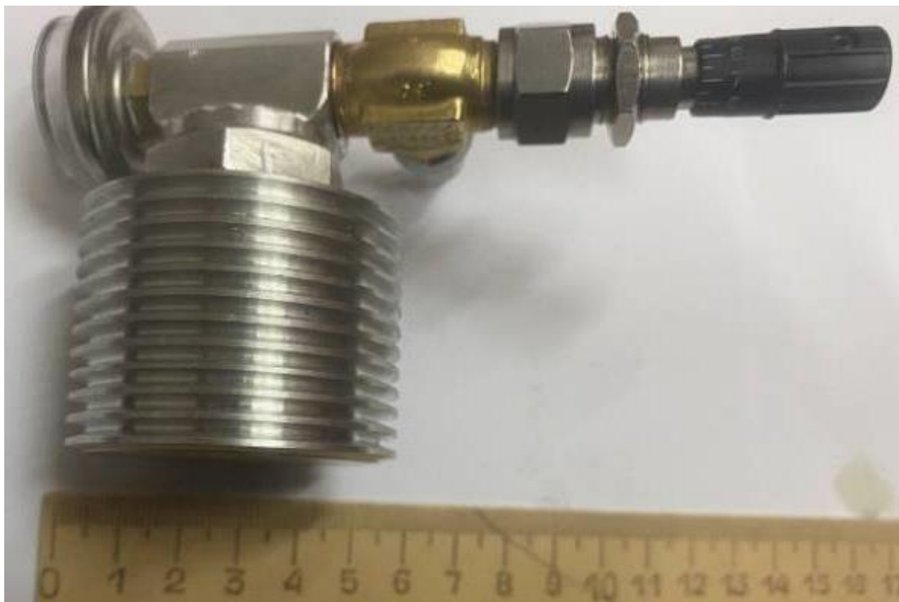
Figure 1. The hydrogen storage device is made from AMg5.
