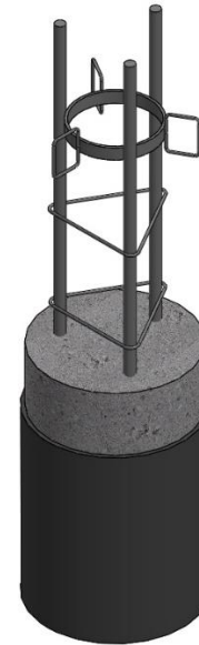
Fig. 3. Reinforcement of pipe concrete pile.
