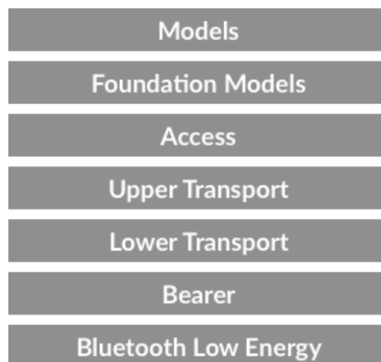
Fig. 5. Bluetooth Mesh architecture
