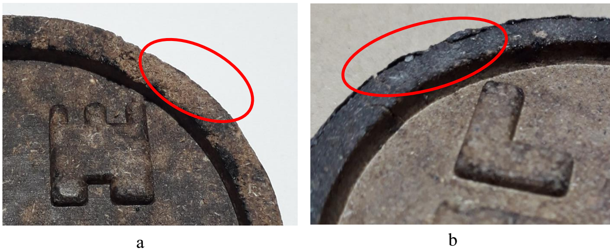
Figure 3.2. Appearance of the product with defects: a – the area of cracking; b - the area of the storm
