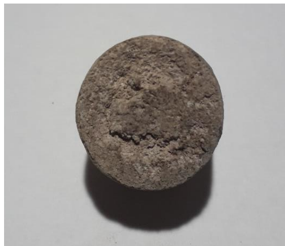
Figure 5.8. Macrostructure of biocomposites modified with sodium sulfate ( \text{Na}_2\text{SO}_4 ):
