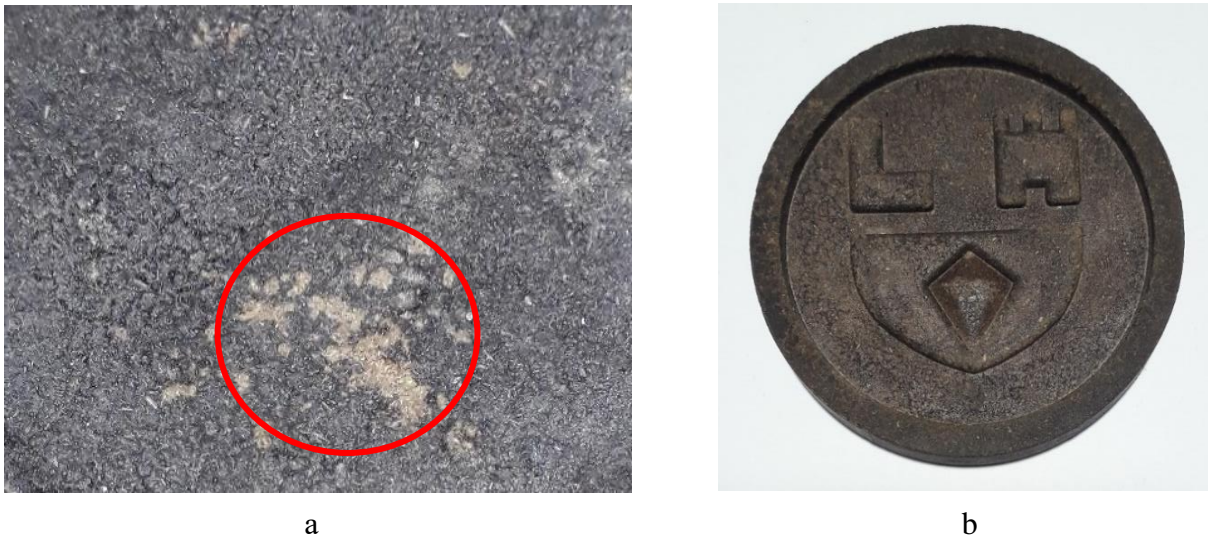
Figure 3.3. Appearance of the product with defects: a – delamination zone; b – lyophobic surface of the biocomposite product
