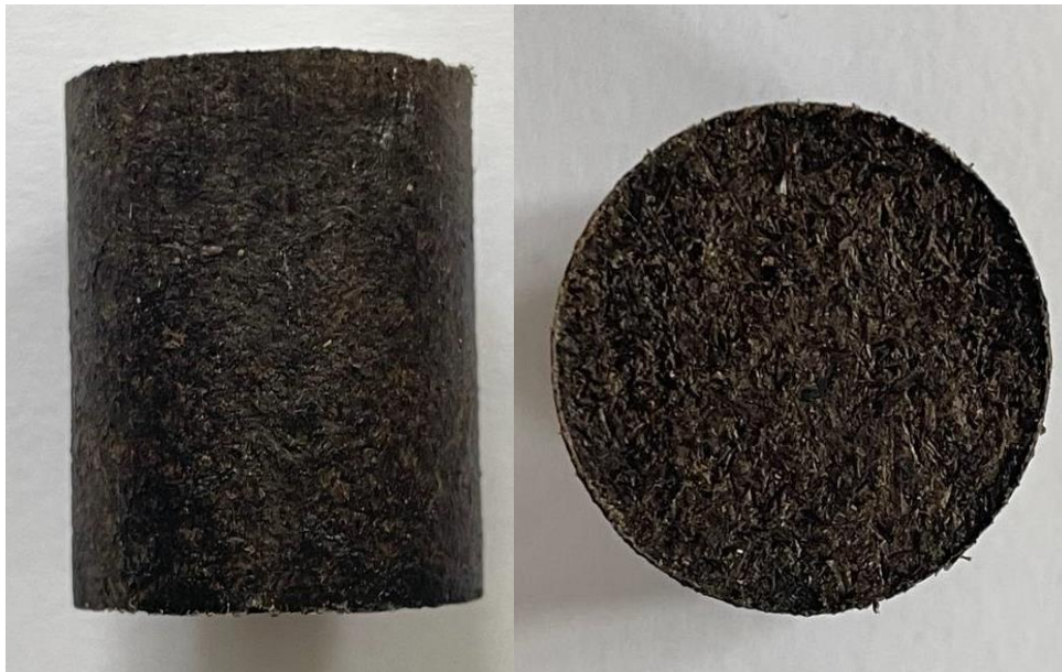
Figure 4.4. The appearance of a biocomposite sample ( \times 2 ) formed by technology No. 2 (Table 4.1)
