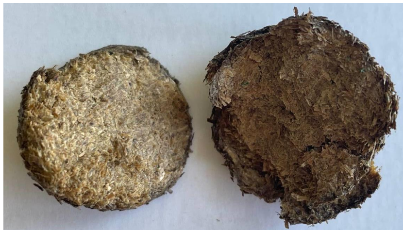
Figure 4.5. The appearance of the fracture surface of biocomposites formed according to modes No. 2 (a) and No. 4 (b)
