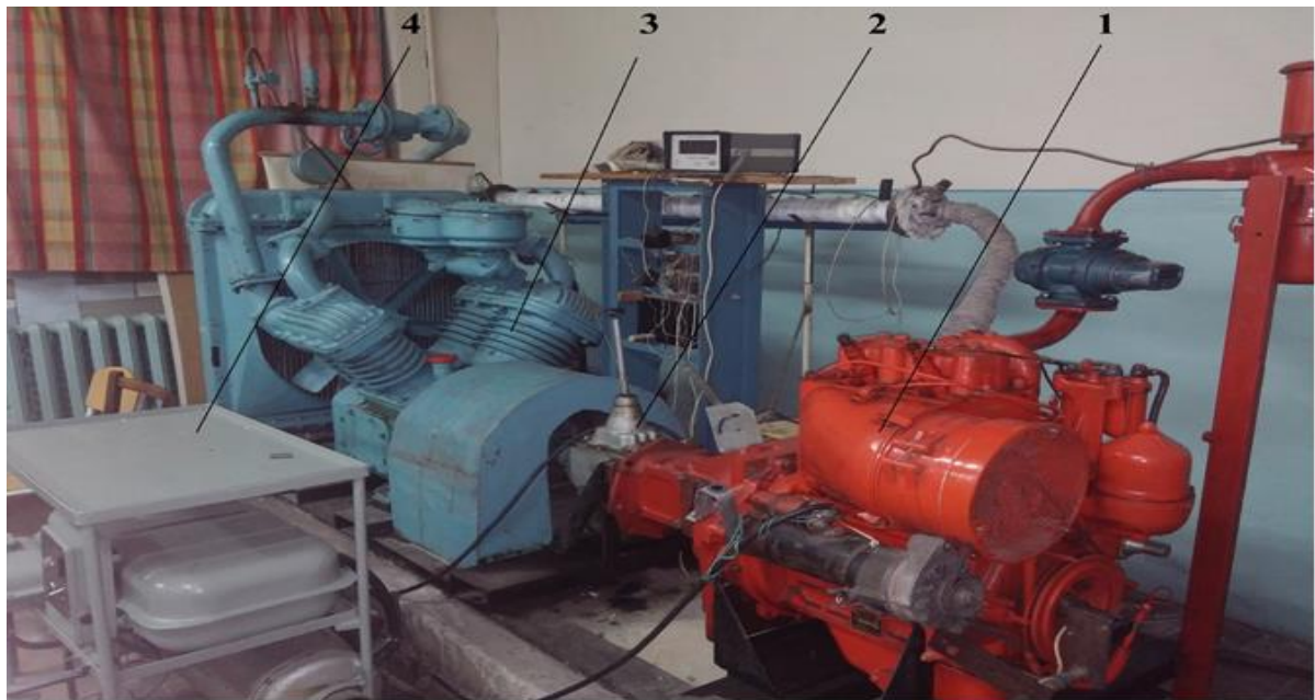
Figure 1. The appearance of the experimental stand based on the D21A1 diesel engine converted to gas for the study of the performance of the engine on alternative gas mixtures.
