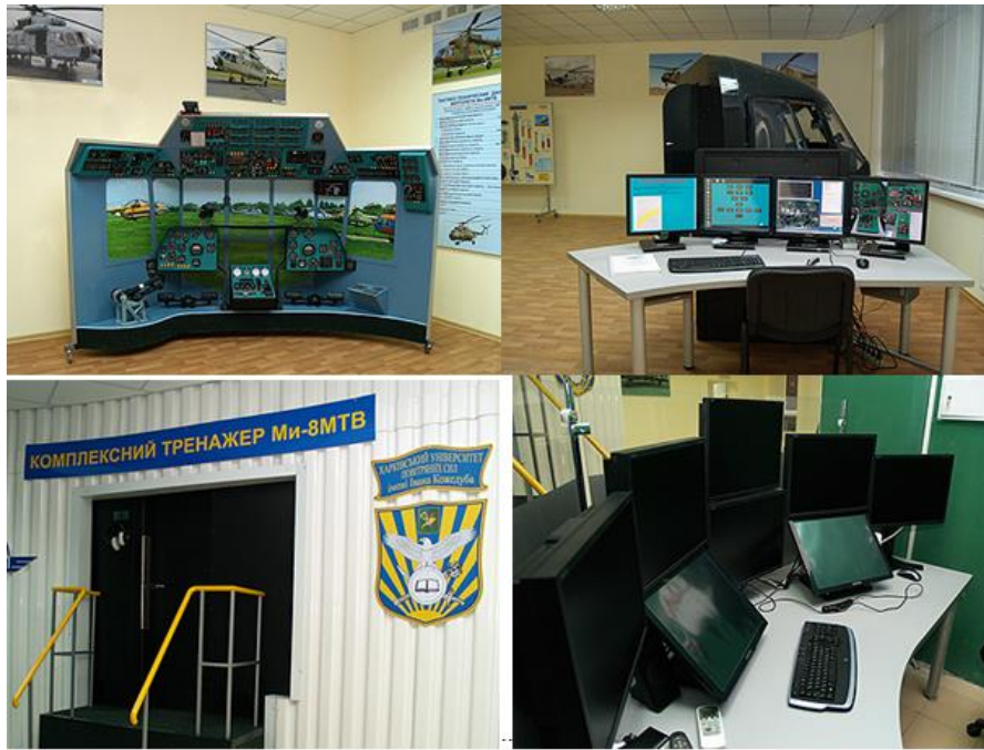
Figure 7. The complex simulator of the «Mi-8 MTB» helicopter.
