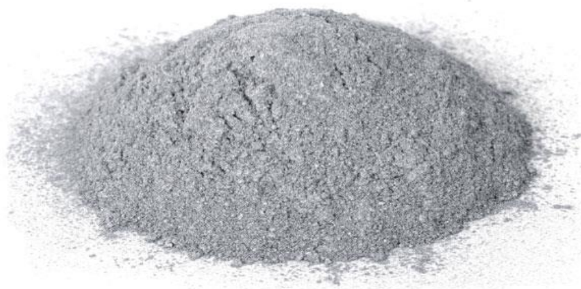
Figure 2. Most metal 3D printing processes start with an "atomized" powder
