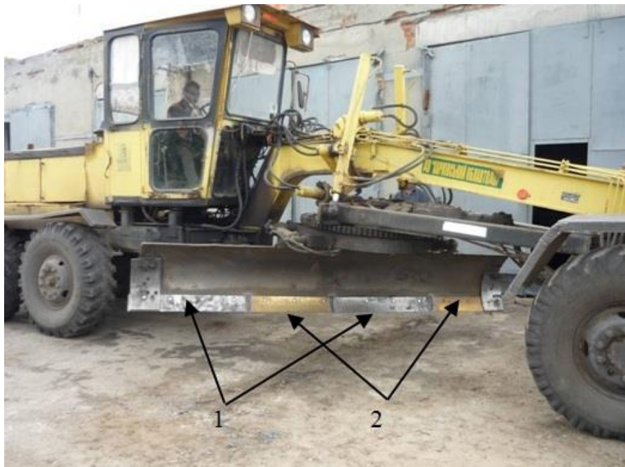
Figure 1. General view of the auto grader DZ-180 with cutting knives hardened by high frequency currents (HFC) (1) and HFC + TiN-Cr 2 N (2)
