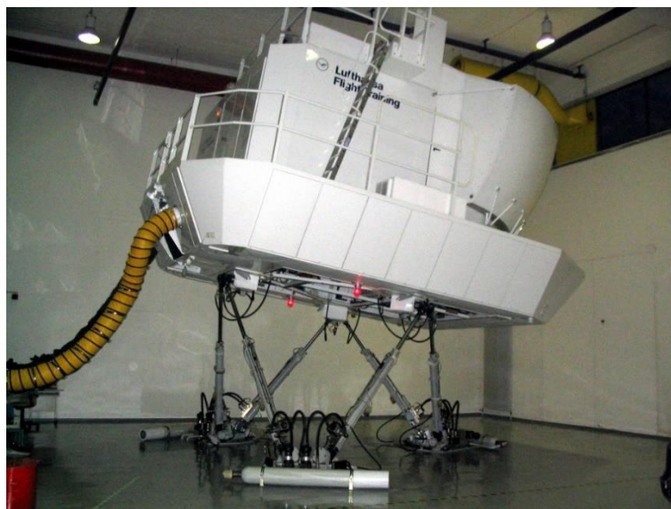
Fig. 1. Full flight simulator with a six degrees-of-freedom motion system
