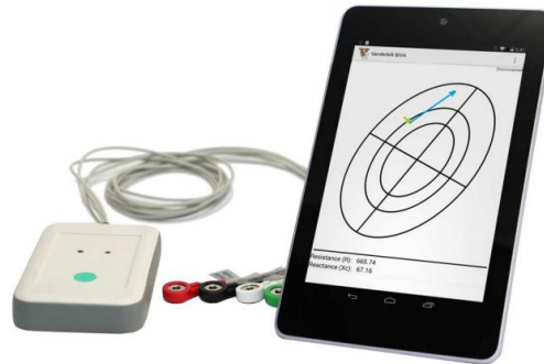
Figure 1. Wireless multifrequency bioimpedance spectrometer (left) and mobile application for data export (right) [5].
