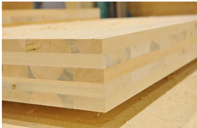
Figure 3. CLT (Cross-laminated timber) [10].
