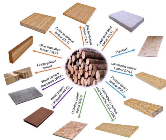
Figure 1. Types of building materials from modified wood [5]
