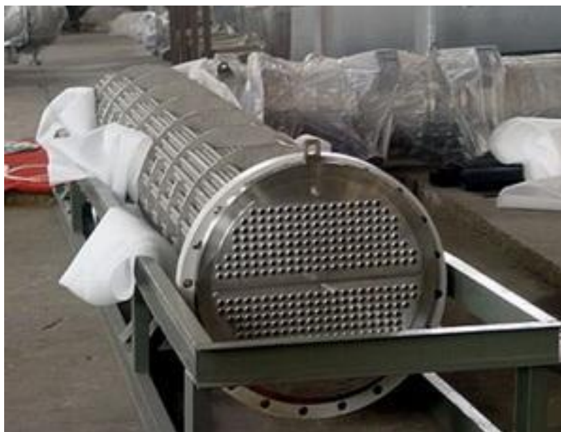
Fig. 1.16. General view of the shell-and-tube heat exchanger
