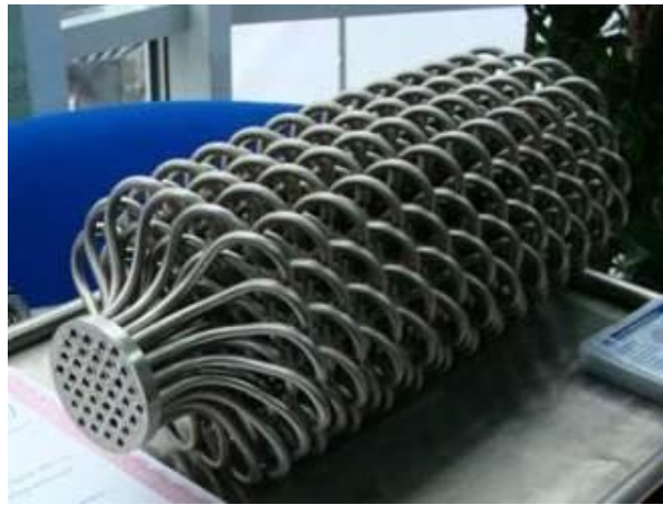
Fig. 1.13. General view of a twisted heat exchanger
