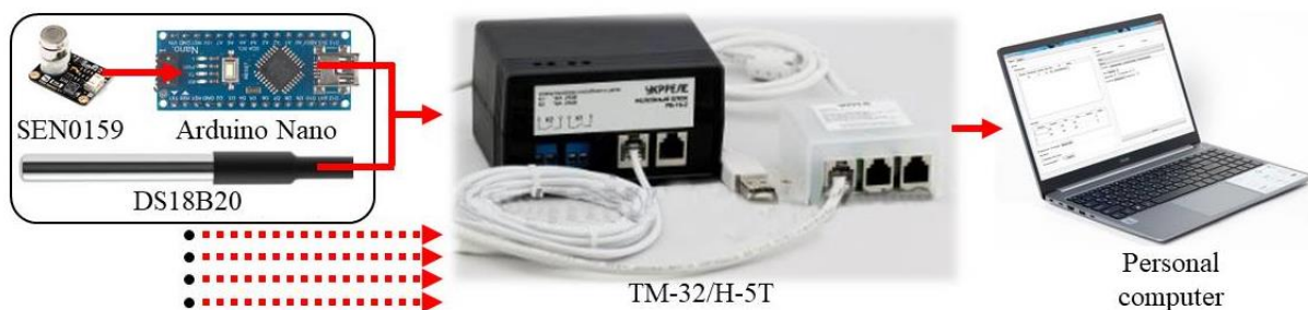
Fig. 2.7. Sensor connection diagram
