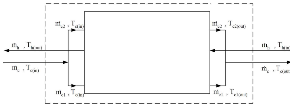
Fig. 1.20. Equivalent circuit of the heat exchanger according to research
