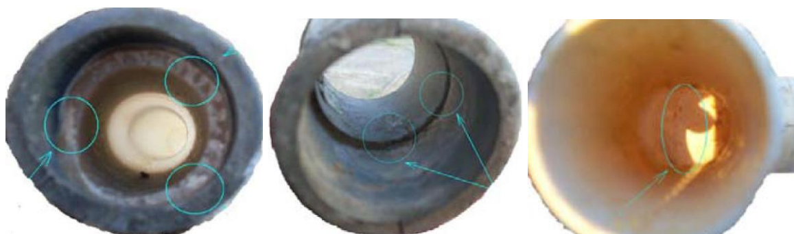
Fig. 4.2. Fragments of mechanical pollution in separate areas of milk duct systems [97]
