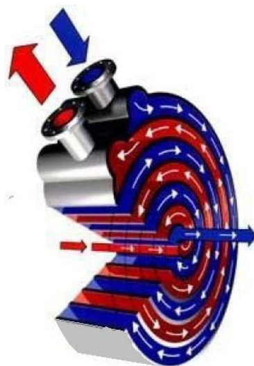
Fig. 1.14. General view of the spiral heat exchanger
