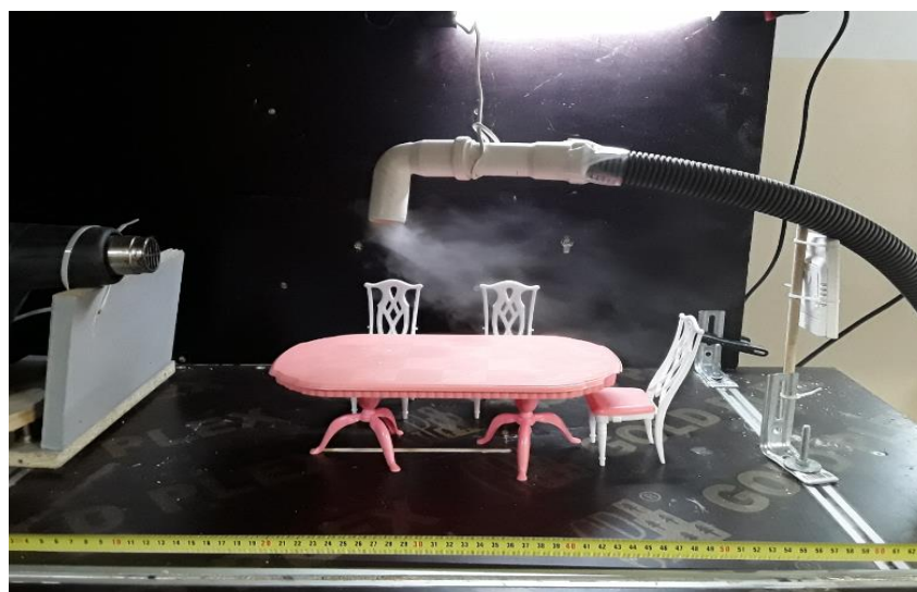
Figure 11. Fog field: V=1.35 – 1.48 m/s, Q=0.832 ml/s (first scenario)
