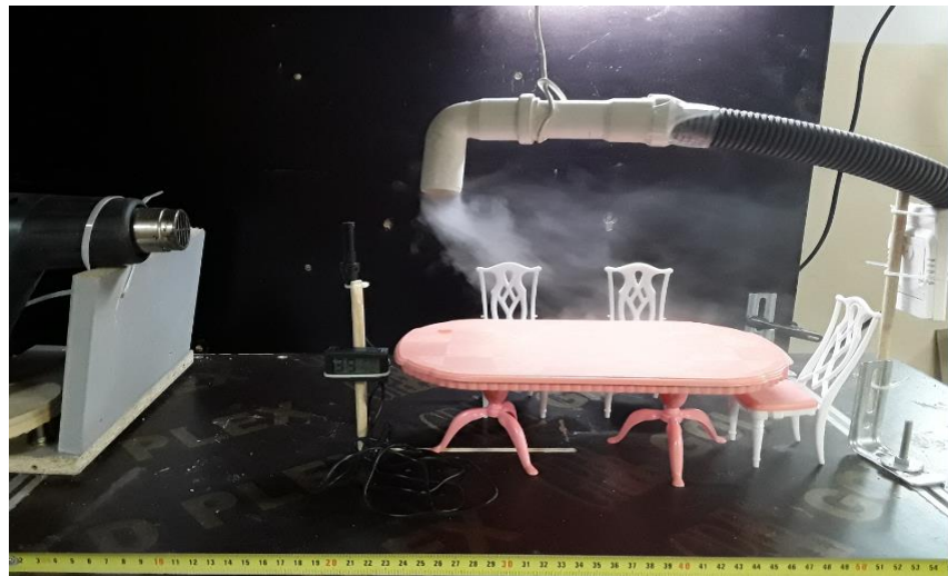
Figure 13. Fog field: V=1.35 - 1.48 m/s. Q=1.167 ml/s (second scenario)
