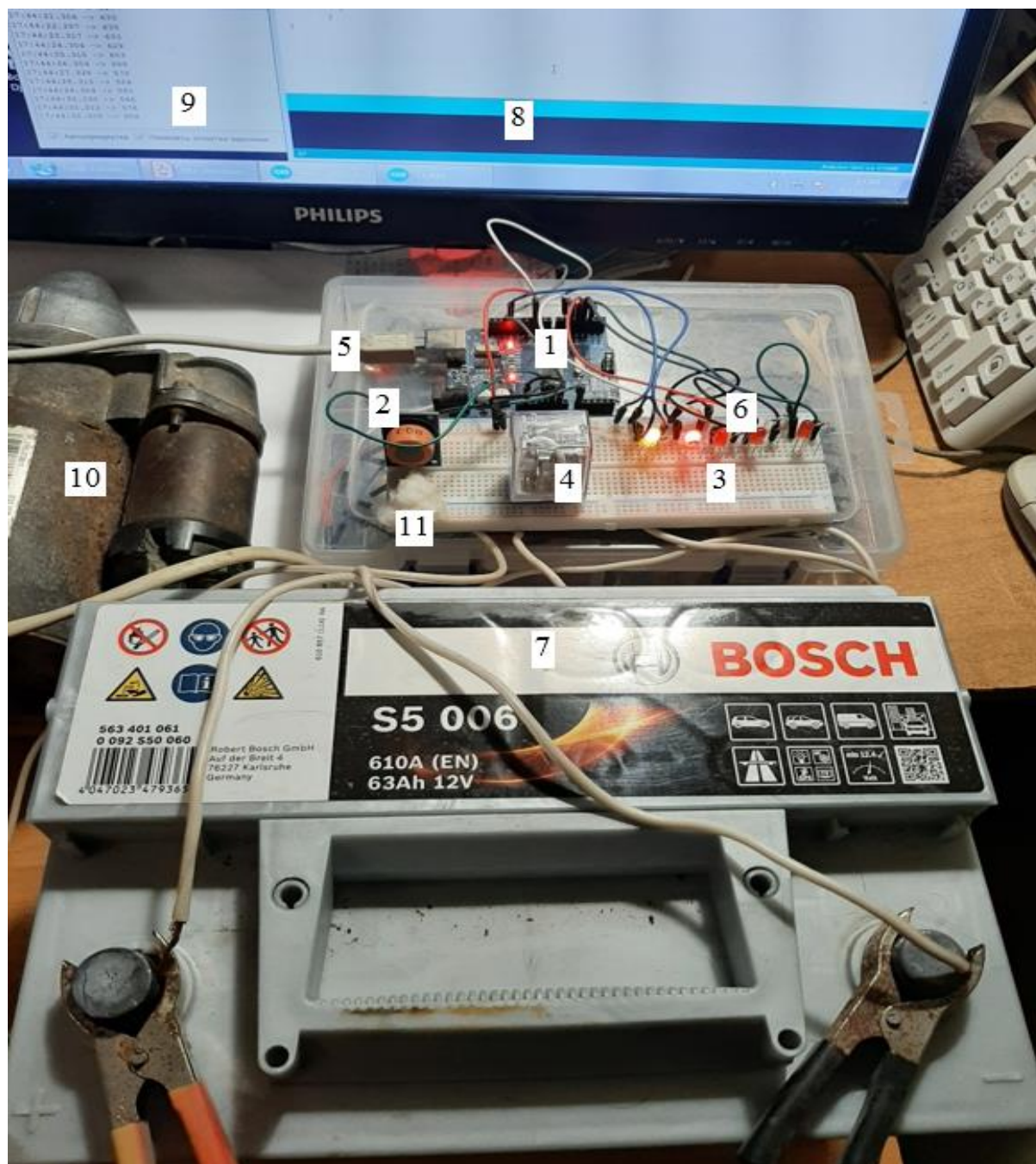
Figure 11. Experimental verification of the blocking device with a car battery and a starter: 1 – Arduino Uno board; 2 – MQ3 sensor; 3 – breadboard; 4 – relay module; 5 – USB cable for connecting to a computer; 6 – five LEDs to indicate the value of the MQ3 signal; 7 – car battery; 8 – Arduino program window; 9 – monitor with signal values; 10 – starter; 11 – cotton wool with alcohol
