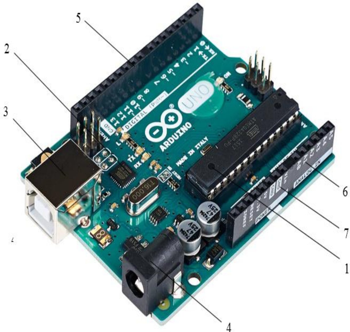
Figure 6. Arduino Uno microprocessor system version R3: 1 – ATmega328P microcontroller; 2 – ATmega16U2 microcontroller; 3 – USB port of the board; 4 – power connector; 5 – 14 digital outputs; 6 – 6 analog outputs; 7 – power outputs
