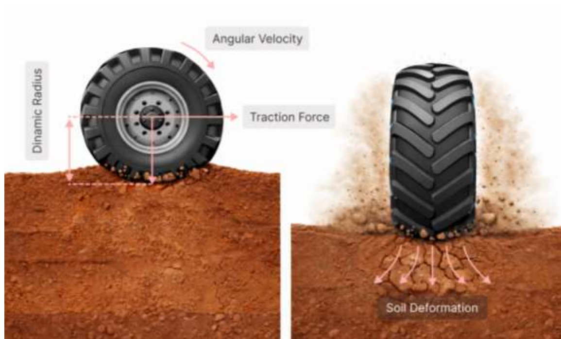
Figure 4. Main parameters in the study of the stress-strain state and the direction of deformations
