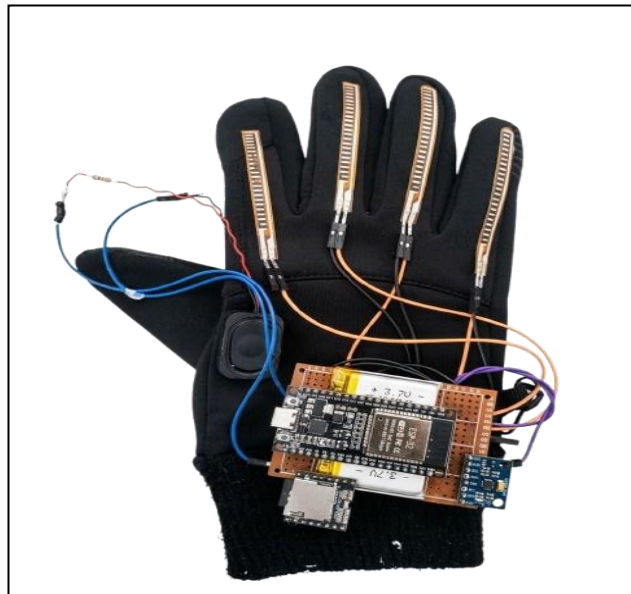
Fig.2 Smart Glove Gesture-to-Voice Message Translation for Mute Persons Source of the figure: author's development
