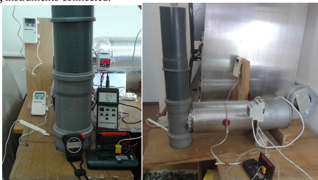
Figure 2. Experimental setup equipped with instruments for measuring temperature and gas-flow velocity. Source of the figure: own illustration
