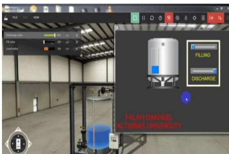
Figure 2. Reservoir emptying procedure within the SCADA system (developed by the author using Factory I/O).
